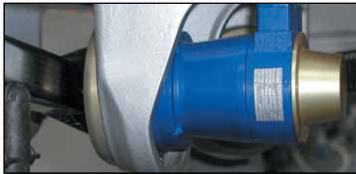
Figure 3. Motor-gearbox drive with carbon lever
