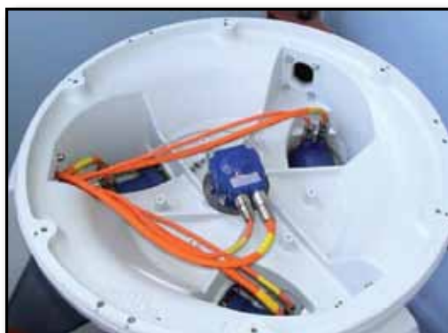
Figure 2. New design using Alpha's TPM motor-gearbox combination
