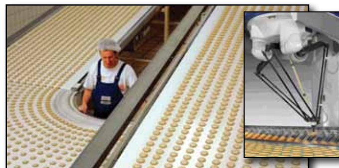
Figure 4. Sigpack Systems Delta Robot in action
