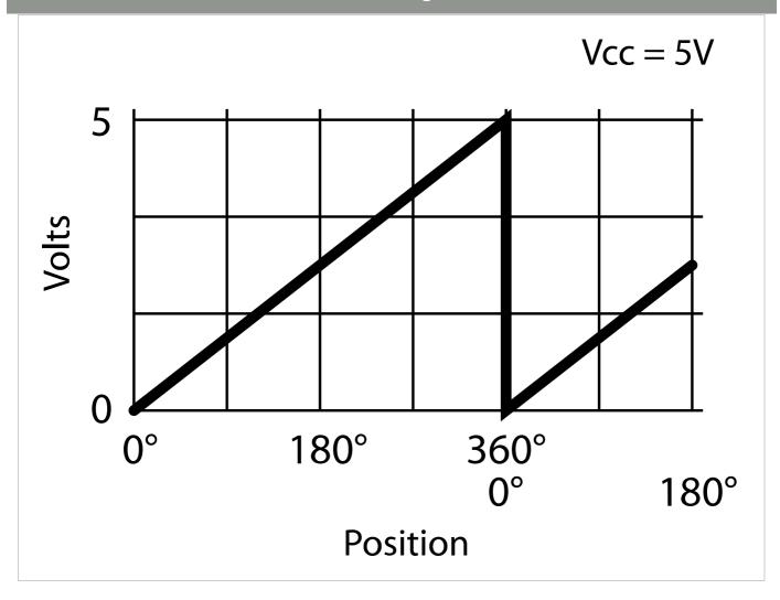
Analog output is only available in 10-bit resolution. The analog output voltage is ratiometric to the power supply voltage and will typically swing within 15 millivolts of the power supply rails with no output load. This non-linearity near the rails increases with increasing output loads. For this reason, the output load impedance should be  $\geq 4.7 k\Omega$  and less than 100pF. The graphs below show the typical output levels for various output loads when powered by a 5V supply.
