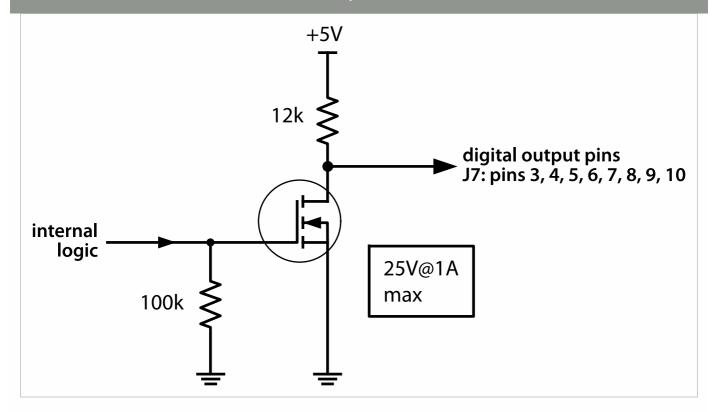
Note: When driving inductive loads, add an external reversed biased diode in parallel with the load to protect the USB4 from damage caused by large voltage transients.
