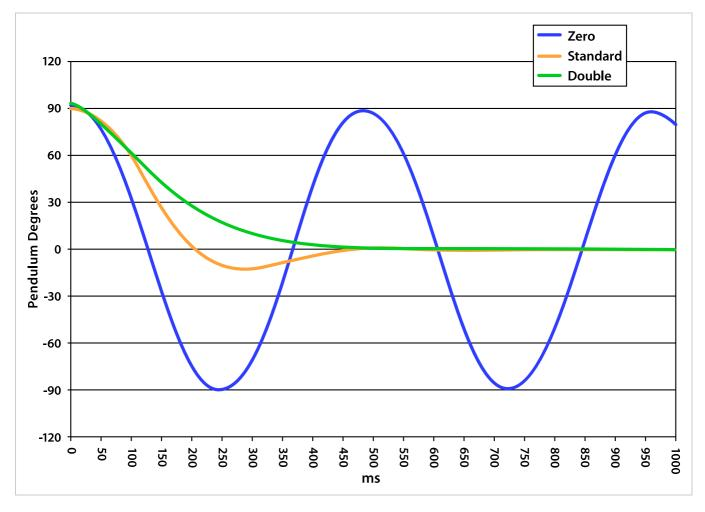
Damping affects settling time and overshoot. Standard damping will fit most applications. Double damping eliminates oscillation but settles to the final position more slowly. Some applications may require double damping to average out cyclic motion such as found in moving vehicles. Damping options can be specified when ordering.
